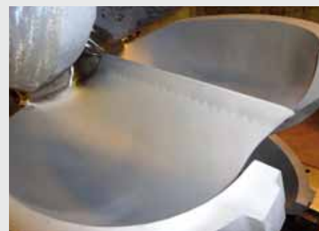
SXH™70-coated Pelton Bucket, Aletsch Mörel, Switzerland
