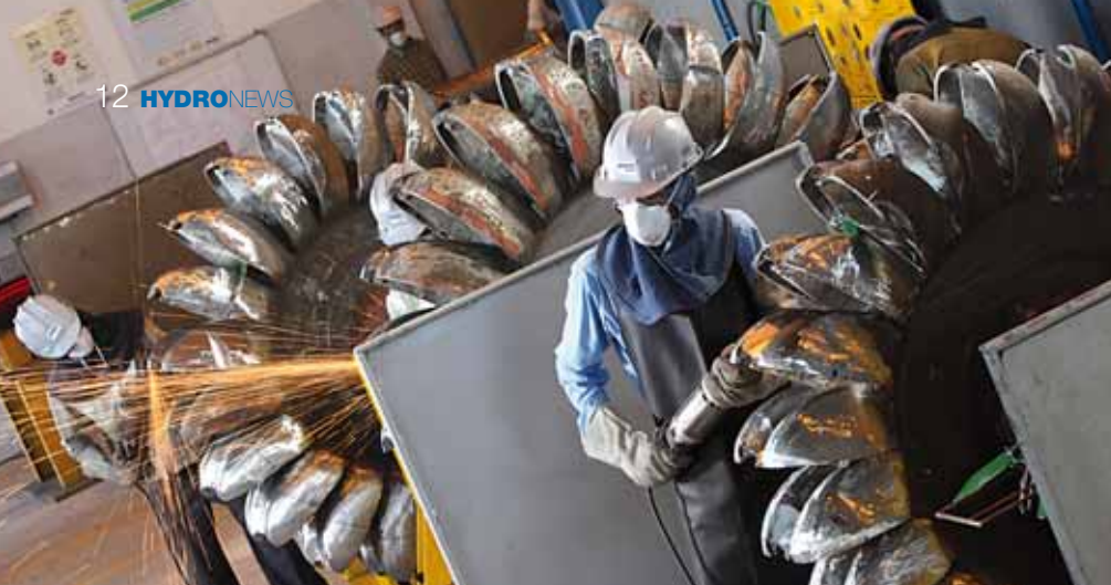
Grinding of Pelton turbine runner at the ANDRITZ HYDRO India Prithla plant
