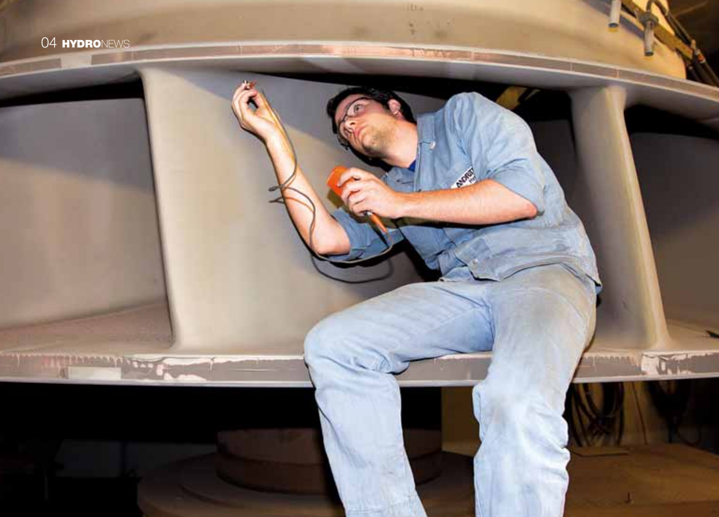
Thickness control of the coating on a Francis runner
