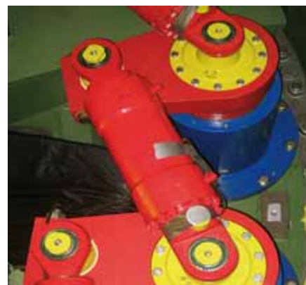
Wicket gate mechanism with individual servomotors
